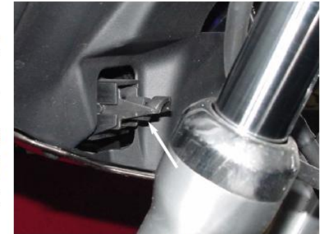
Base setting adjustment screw
